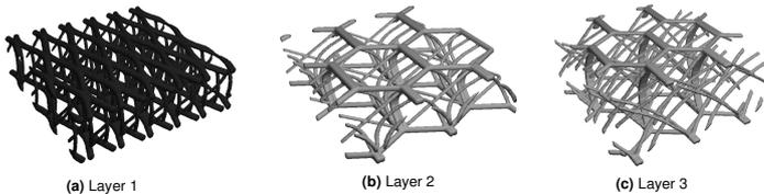
Fig. 4: Modeled layers of the thermal collector
